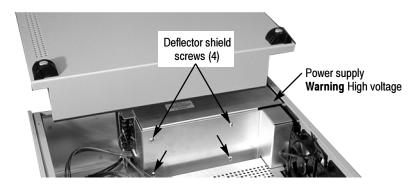
Figure 5-7: Remove the power supply shield
