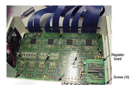
Figure 5-8: Remove the logic board from the chassis
