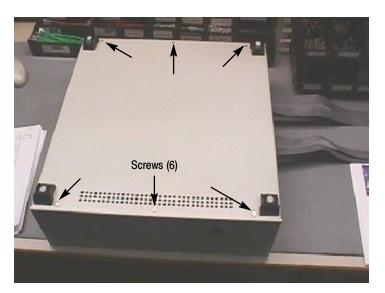
Figure 5-11: Remove the attaching screws
