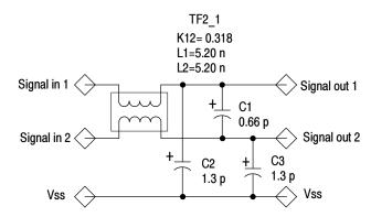
Figure 3-3: ZIF electrical load model for typical signals
