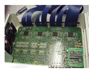
Figure 5-13: Place logic board in the chassis
