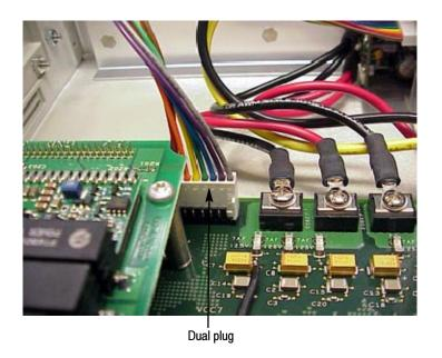
Figure 5-19: Attach the power supply dual plug
