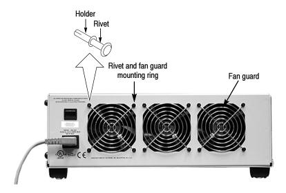
Figure 5-25: Back of the preprocessor unit
