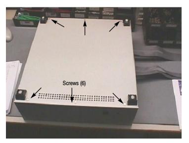
Figure 5-22: Remove the bottom cover
