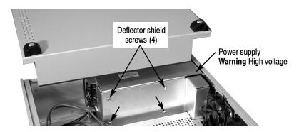
Figure 5-15: Attach the power supply shield
