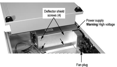
Figure 5-23: Remove the bottom cover
