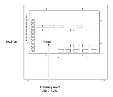
Figure 1-2: Jumper locations on the preprocessor unit
