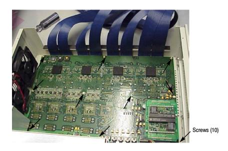
Figure 5-14: Attach the logic board to the chassis
