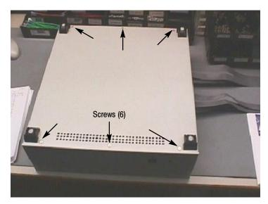
Figure 5-2: Remove the attaching screws
