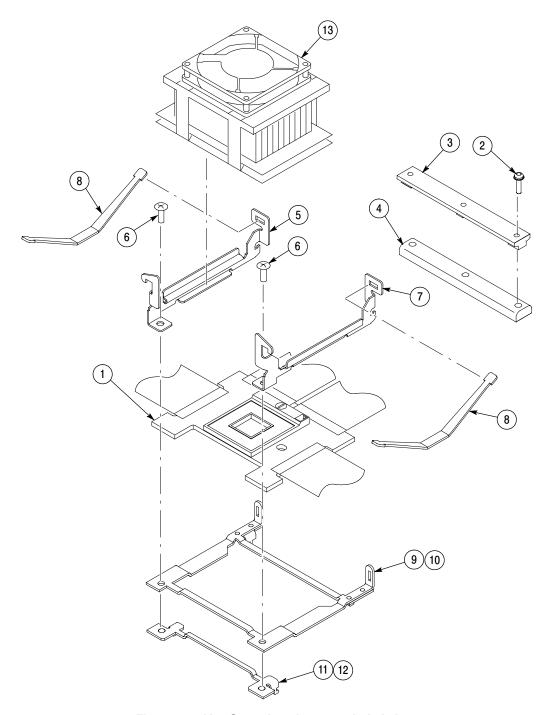
Figure 6-1: IA32G8 probe adapter exploded view
