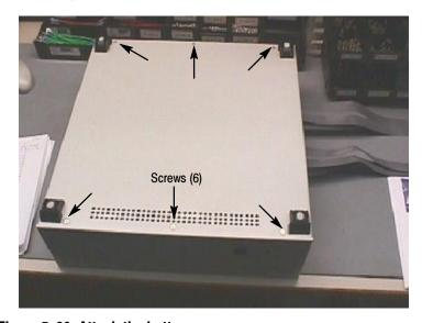
Figure 5-20: Attach the bottom cover
