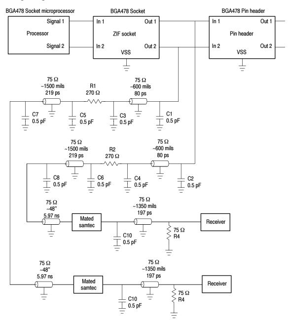
Figure 3-1: Electrical load model for typical signals
