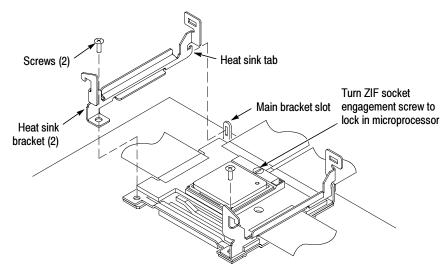
Figure 1-7: Connect the 478-Pin Socket microprocessor and the heat-sink brackets
