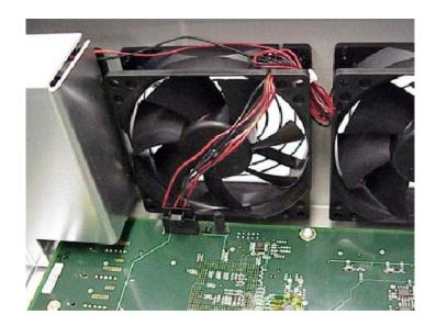
Figure 5-3: Remove the fan plug
