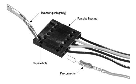
Figure 5-24: Remove the pin connectors
