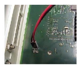
Figure 5-17: Attach the LED cable to the Logic board
