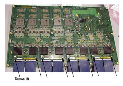
Figure 5-12: Attach the cables to the logic board
