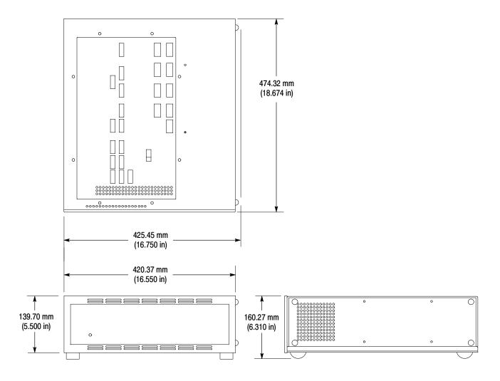
Figure 3-7: Dimensions of the preprocessor unit
