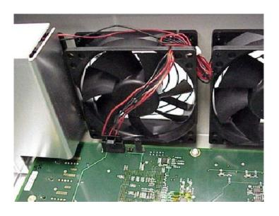
Figure 5-16: Attach fan plug
