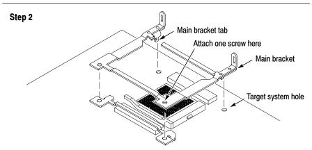
Figure 1-5: Install the front and main-brackets
