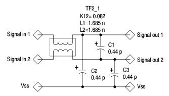
Figure 3-2: Pin header electrical load model for typical signals
