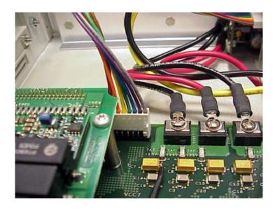
Figure 5-6: Remove the power supply dual plug
