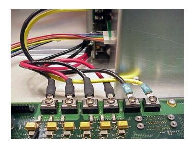
Figure 5-5: Remove power supply cables
