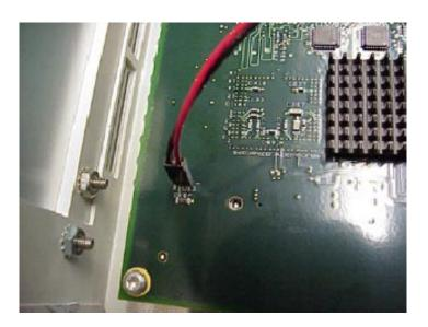
Figure 5-4: Remove the LED cable
