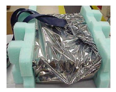
Figure 1-13: Place the end caps on the preprocessor
