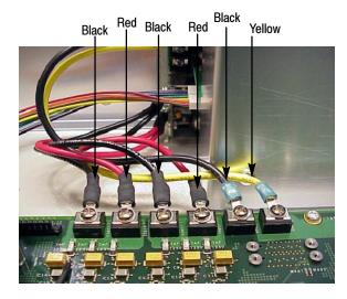
Figure 5-18: Attach the power supply cables
